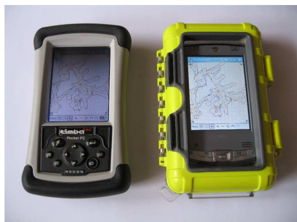
Fig. 3: TDS Recon Outdoor PDA (left) and Palmcase Armor waterproof case (right).
