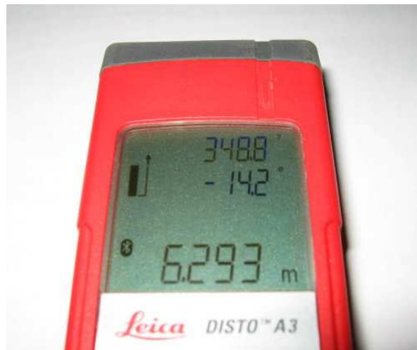
Fig. 2: Leica Disto with compass and clinometer readings added to the standard display.
