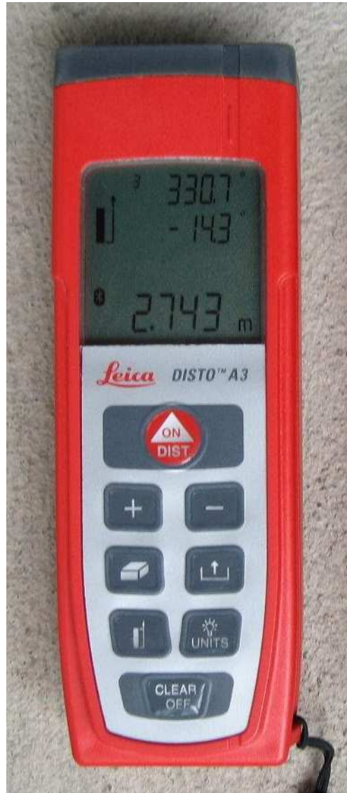
Fig. 1: The DistoX with azimuth, inclination, and distance readout.
