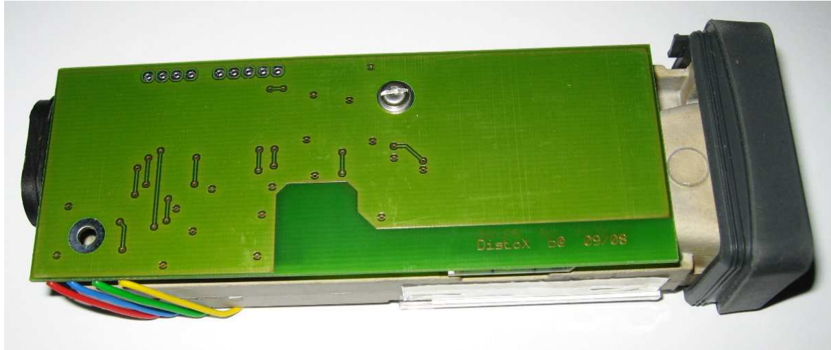
Fig. 3: Upgrade board mounted to the chassis of the Disto
