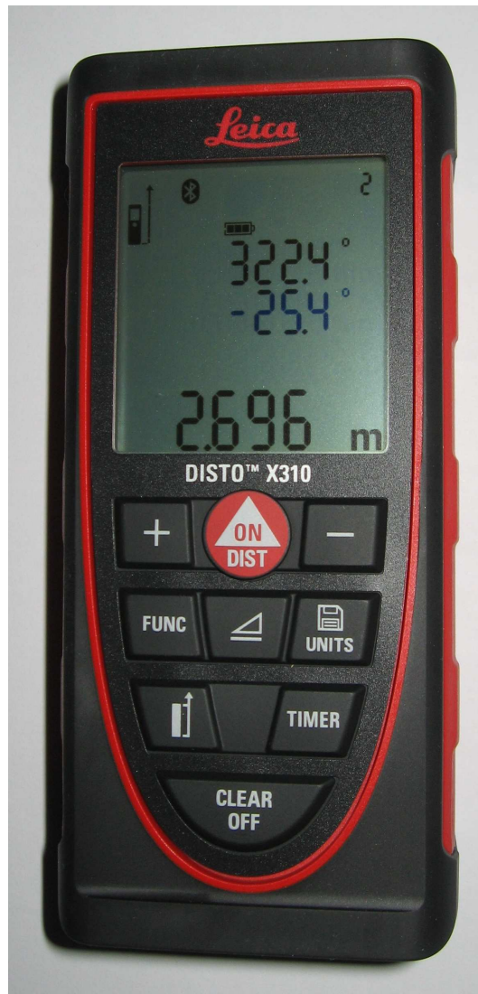
Figure 1 - The DistoX2 with azimuth, inclination, and distance readouts.
