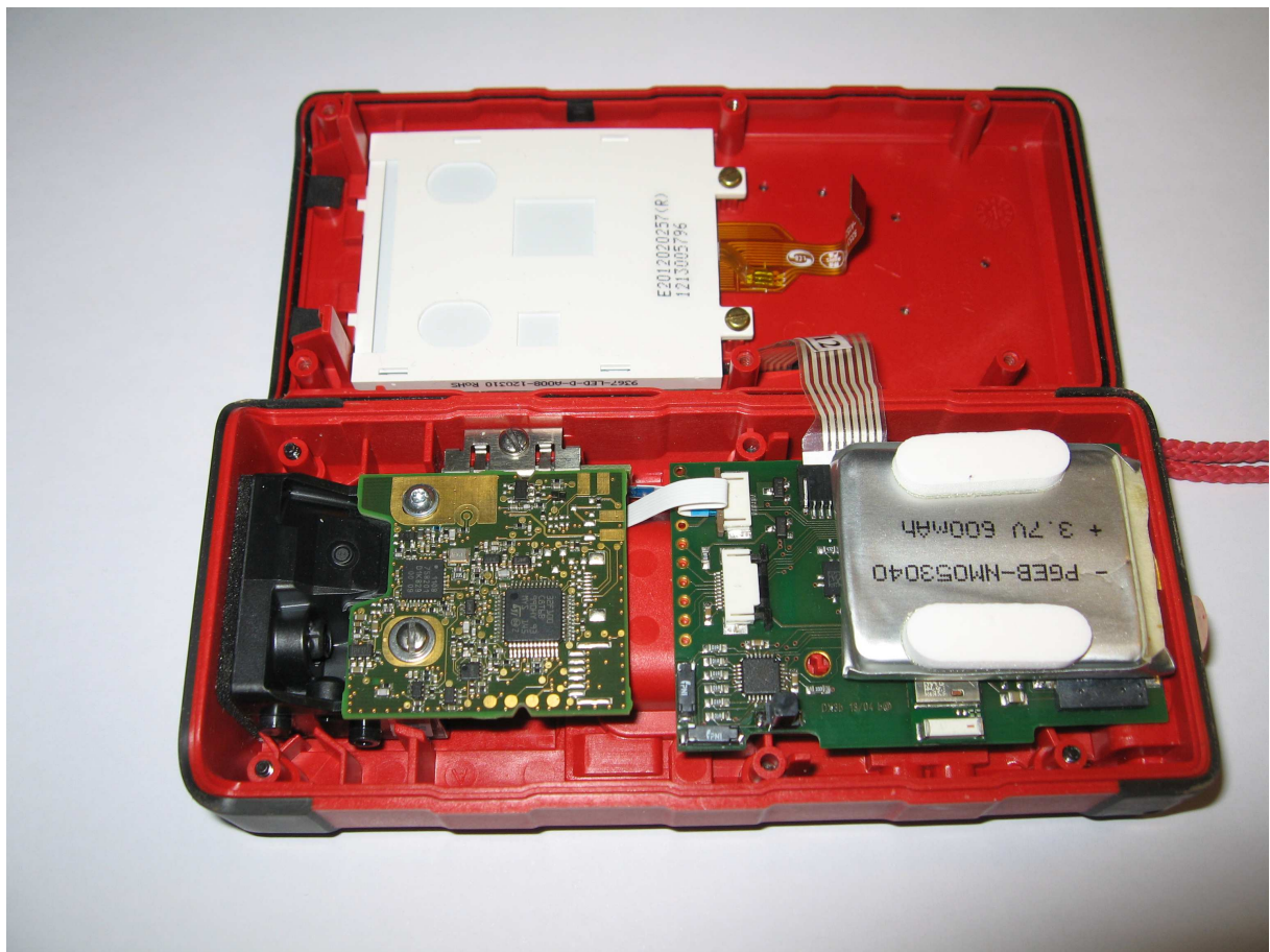
Figure 3 - Upgrade board and LiPo battery mounted inside the Disto
